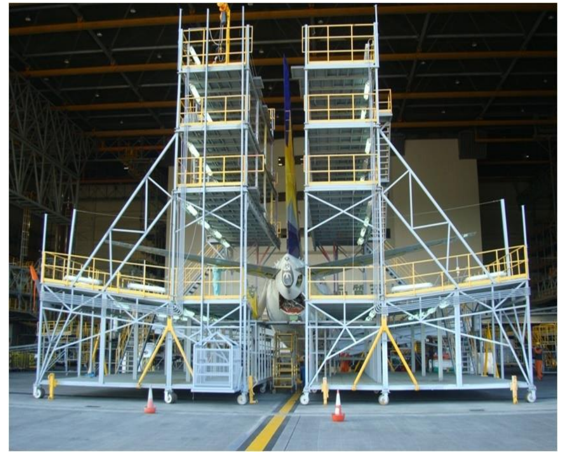
Aircraft Maintenance Platform
