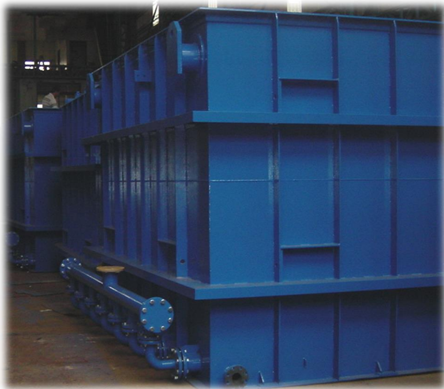
Waste Water Treatment Tank
