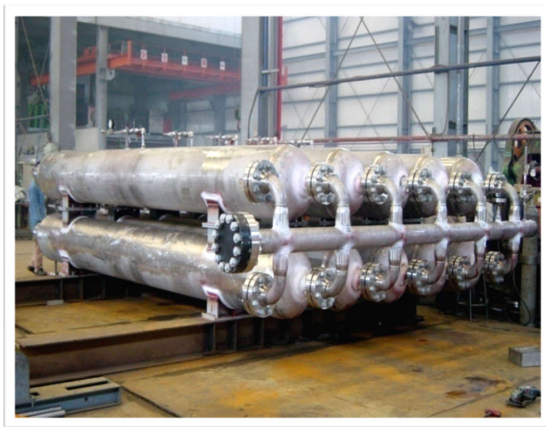
HTTF Ultra High Pressure Storage Tank Test Pressure : 320 kg/cm 2
