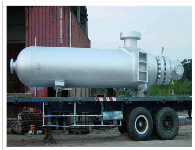
High Pressure Heat Storage Accumulator Test Pressure : 215 kg/cm 2
